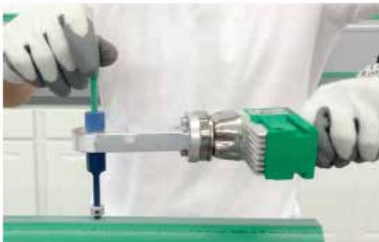
Picture no. 47: Inserting reparation tools
