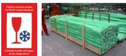
Picture no. 6: Appearance of unit packages in transport package
