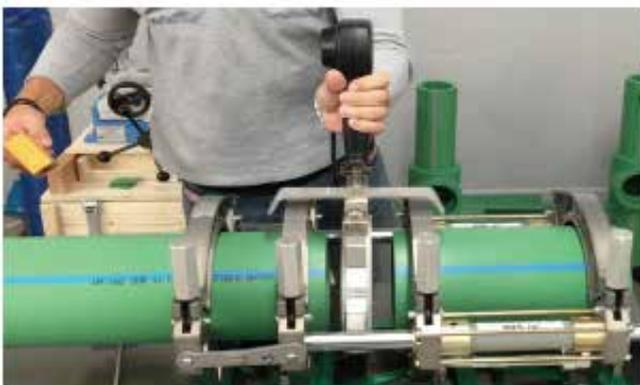
Picture no. 43: Insertion of the heating plate
