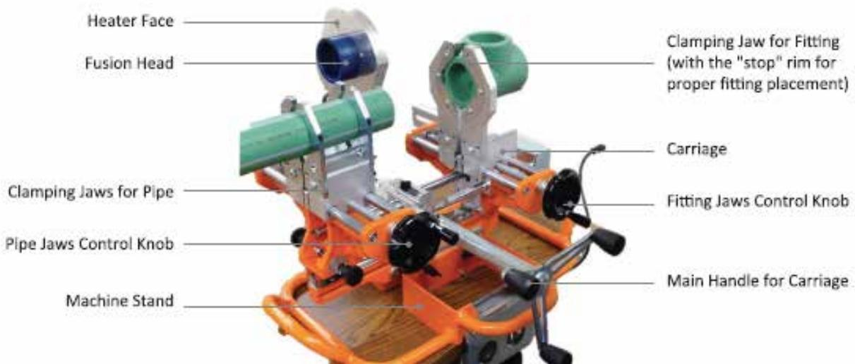
Picture no. 35: Appearance stationary welding machines
