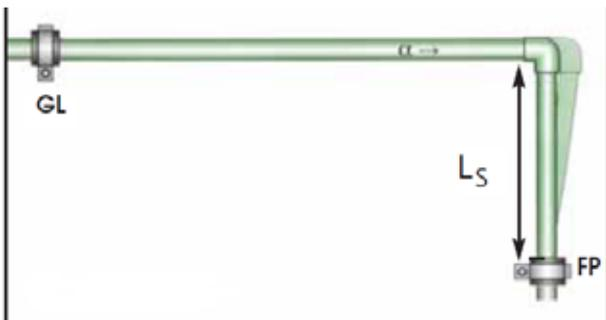
Picture no. 60: Display of the correct acceptance of longitudinal dilatations by changing the direction, where GL is a plain bearing (support), and FP fixed bearing (fixed support), while  $L_s$  is required length of change direction.
