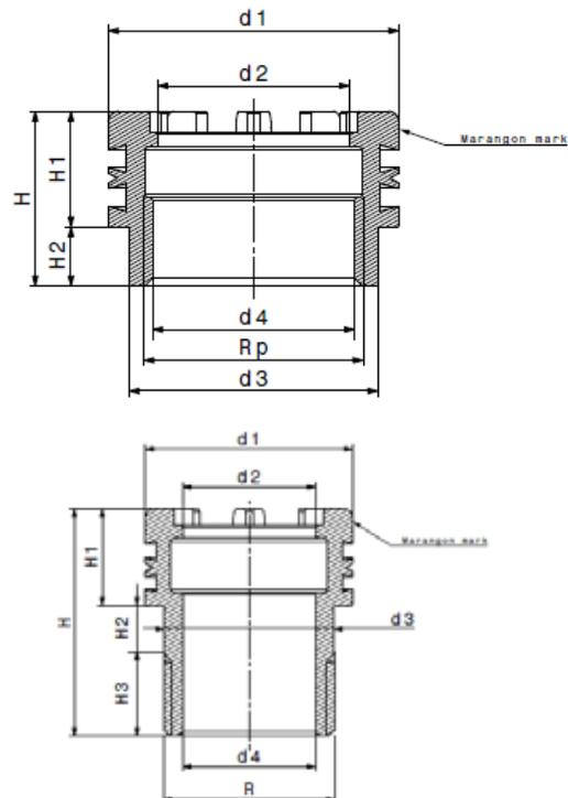
Picture no. 50: Technical drawings of UN/SN inserts
