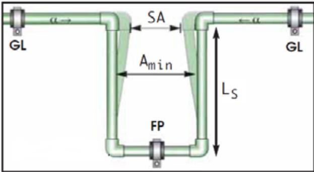
**Picture no. 61:** Display of the correct acceptance of longitudinal dilations through the lever, where the GL is a plain bearing (support), FP-fixed bearing (support),  $L_s$  - required direction change direction,  $A_{min}$  - width of tube port lire,  $SA$ - safety clearance
