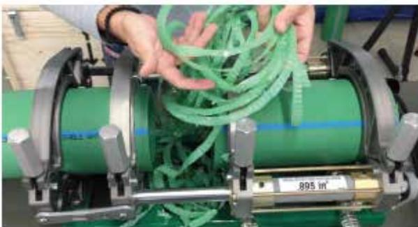
Picture no. 42: A method of processing the ends of the tube
