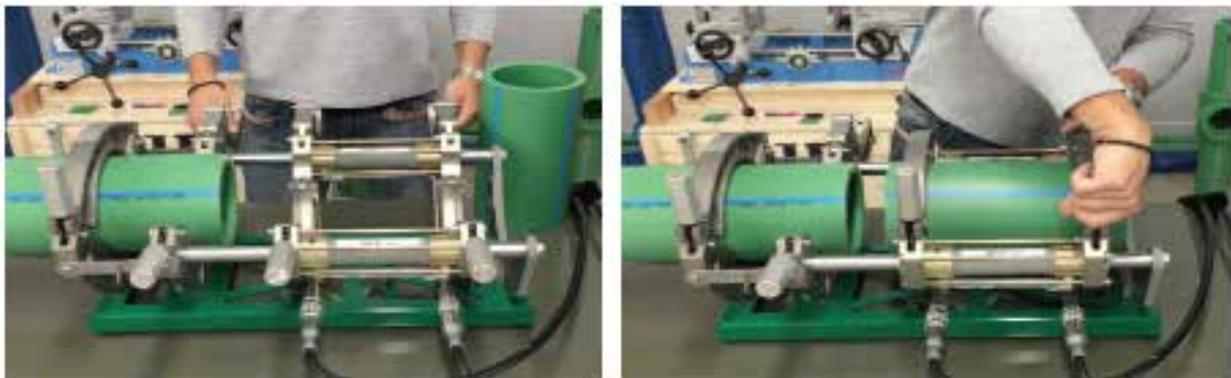
Picture no. 41: Fixing the pipe with jaws
