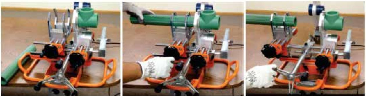
**Picture no. 37:** Pipe and fitting alignment procedure
