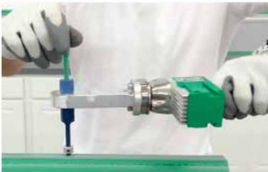
Picture no. 47: Inserting reparation tools
