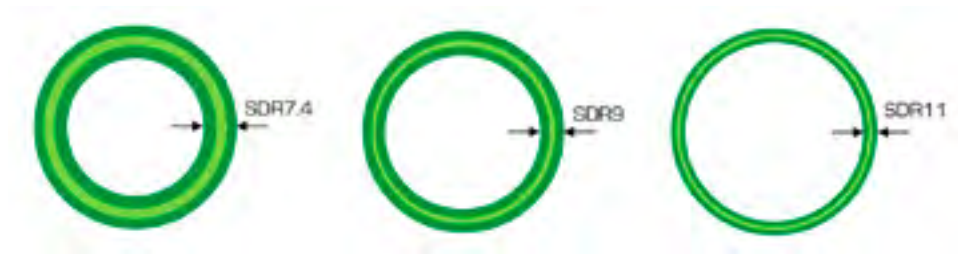
The SDR of the pipe is important as it is used as a design parameter of the pipe. The lower the SDR number, the thicker the pipe wall. A thicker wall increases the pipe's ability to hold pressure.
