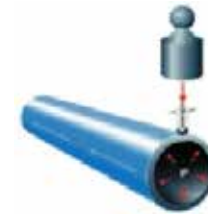
Point load test according to dr. Hessel
