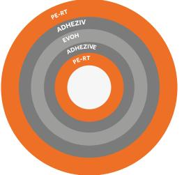
EVOH layer is in the middle of the pipe so it is fully protected from wear and moisture during transport and construction which ensure the full efficiency of EVOH oxygen barrier during the long period e.g. proposed service life of pipe.
