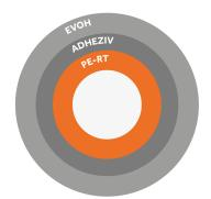
Outer layer of pipe is made of EVOH. Therefore, EVOH is directlly exposed to wear and humidity. Oxygen impermeability will decrease with humidity increas.
