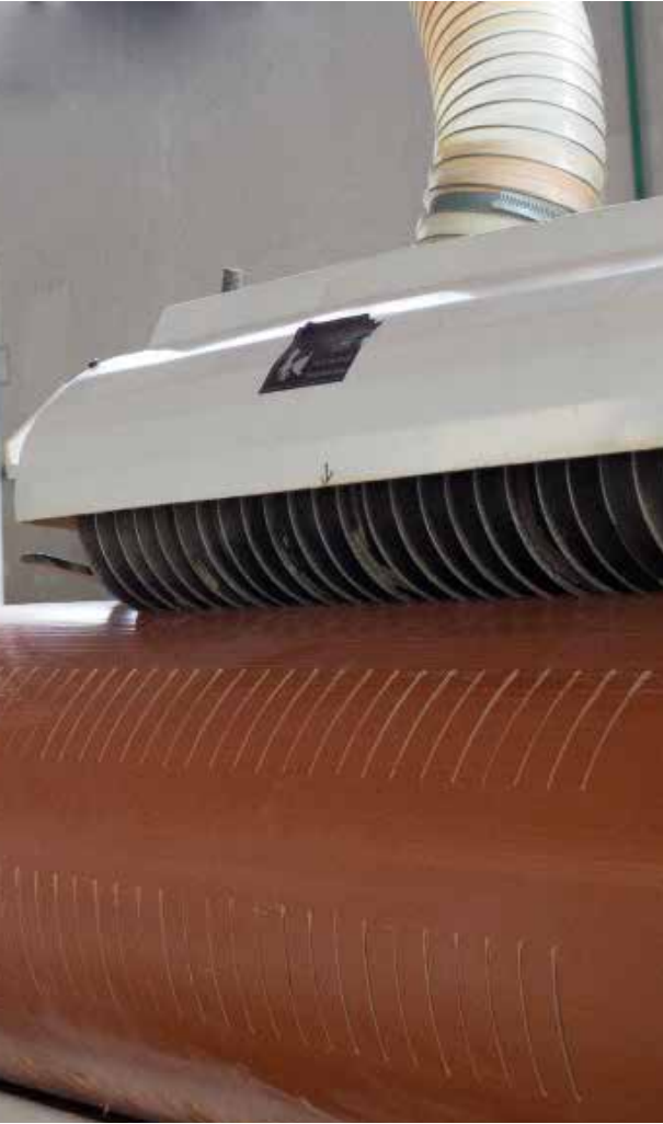
The method of producing perforations in the PVC pipes
