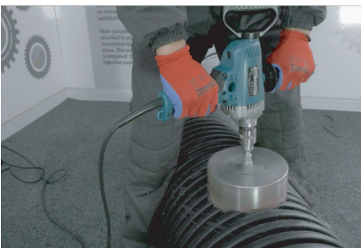
4. Drilling holes with crown saw
