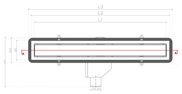
NOTE: Drains in length of 300,450 i 550 come in package with two sets of legs for adjusting of height. Drains in length 650,750 i 850 come in package with four sets of legs for adjusting of height.
