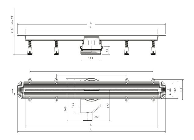
Thanks to universal solution for adjustment height of drain (DN 110mm cuttable reducer) EVO ULTRA THIN shower drain have possibility of installation in both renovation and new building bathroom projects. Minimal installation height is 77mm and maximum is 110mm which fulfills all requests of modern buildings. Height adjustment legs enables extra security during installation and use.
