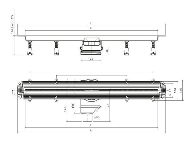
Thanks to universal solution for adjustment height of drain (DN 110mm cuttable reducer) EVO ULTRA THIN shower drain have possibility of installation in both renovation and new building bathroom projects. Minimal installation height is 77mm and maximum is 110mm which fulfills all requests of modern buildings. Height adjustment legs enables extra security during installation and use.
