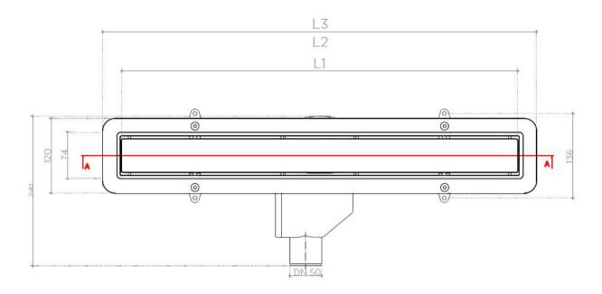
NOTE: Drains in length of 300, 450, 550 and 650 come in package with two sets of legs for adjusting of height. Drains in length 750, 850 and 950 come in package with four sets of legs for adjusting of height.
