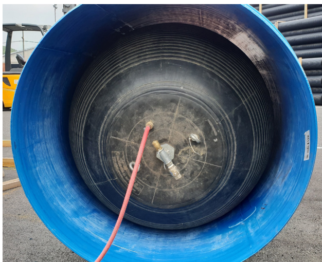
Balloons for testing the tightness of SPIROPIPE pipes
