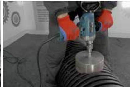
4. Drilling holes with crown saw
