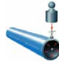
Point load test according to dr. Hassel
